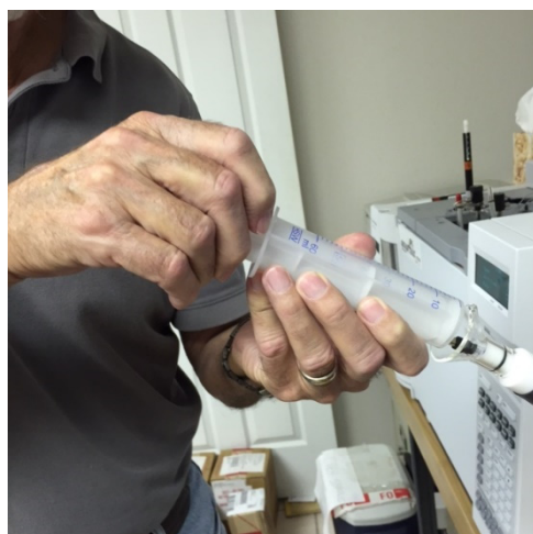
Figure 11. Whole air fraction collection process of high-impact odorants from the sniff port for offline odor assessment.
