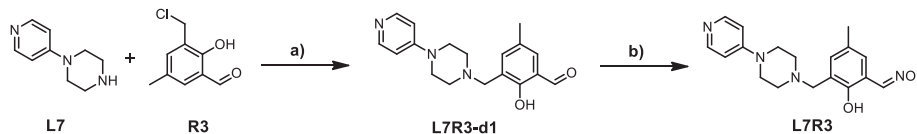
Scheme 1. Preparation of conjugates L7R3 . Conditions and reagents: a) DCM, NEt 3 , r.t. 81%; b) HONH 2 HCl, NaOAc, EtOH/DCM, 76%.
