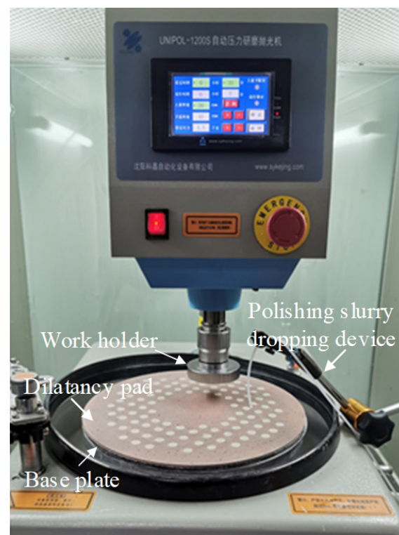
Figure 3. The experimental device of C-SDP.
