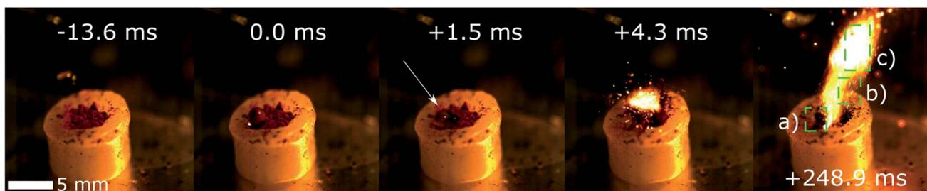
Fig. 5 Drop tests on neat paraffin wax pellet with a 10 mg of Co(Alm)<sub>2</sub> located in a hole in the center, using WFNA as the oxidizer. The location of the first ignition is marked with the white arrow. (a) Burned paraffin and HMOF. (b) Burning HMOF powder. (c) Paraffin flame. Full sequence available in ESI.†
