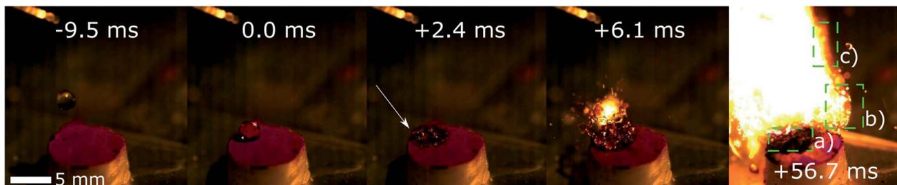
Fig. 4 Example of an ignition drop test on a FR5560 wax pellet covered with a thin 10 mg layer of Co(Alm)<sub>2</sub> (configuration II), using WFNA as the oxidizer. The location of the first ignition is marked with the white arrow. (a) Burned paraffin and HMOFs. (b) Burning HMOF. (c) Paraffin flame. Full sequence available in ESI.†
