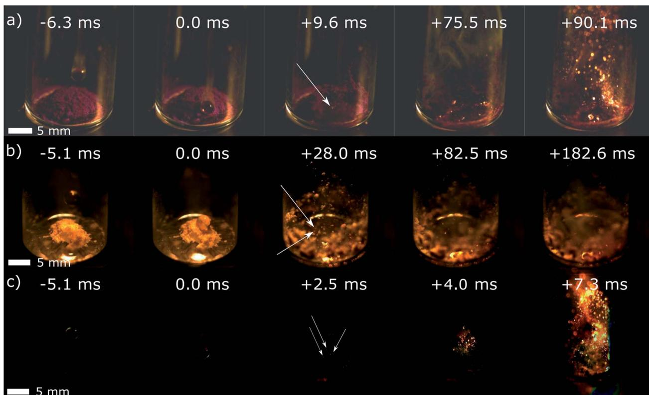
Fig. 2 Droplet ignition tests on (a) pure Co(VIm)<sub>2</sub>, (b) pure Zn(VIm)<sub>2</sub>, and (c) pure Co(AlIm)<sub>2</sub> using *ca.* 10 mg of HMOF powder samples and WFNA as the oxidizer. The location of the first ignition is marked with the white arrow. Picture in (c) were digitally modified to remove reflections on the glass vial. The original videos are available online as ESI.†
