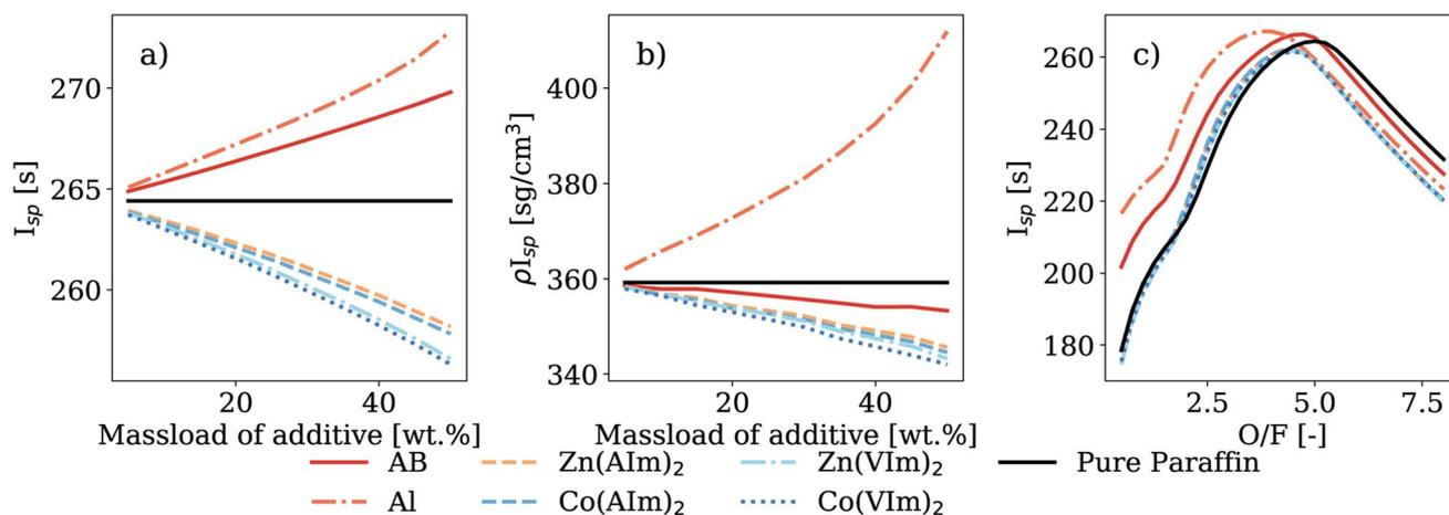
**Fig. 7** (a) Specific impulse as a function of the mass load of additive in a paraffin-based fuel matrix at the optimal O/F ratio, (b) density specific impulse as a function of the mass load of additive in a paraffin-based fuel matrix and (c) theoretical performance at 20 wt%, as a function of oxidizer-to-fuel ratio. Calculated using WFNA as the oxidizer.
