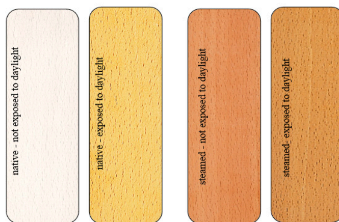
Figure 2. View of beech wood: native before and after exposure (left), steamed before and after exposure (right).
