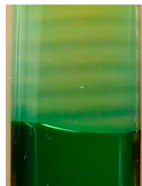
Figure 1. Visible image of a single-head spin mode in the frontal polymerization of a diacrylate with bromophenol blue as an indicator. The alternating green and yellow horizontal patterns in the wake of the spin head are the tracks left by the spiraling hot spot. Tube diameter = 125 mm.
