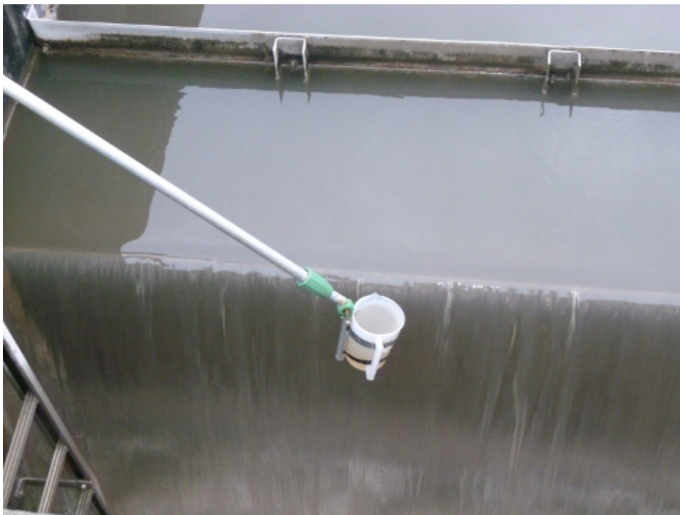
Figure 2. Sampling at the waste water treatment plant after the grid collector (waste water treatment plant Germany). Click here to view larger image.
