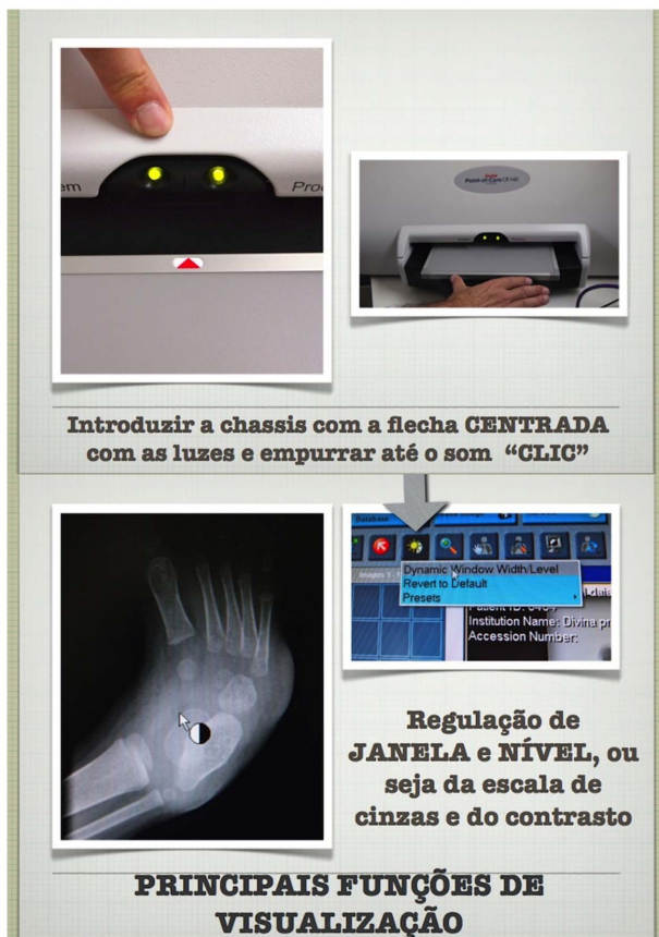
Figure 3. Extract from the training course. Note: This extract from the training course in Portuguese, the national language in Angola, shows how to initiate the system (upper images), and how to choose functions to optimise X-ray visualisation (lower images). doi:10.1371/journal.pone.0073939.g003
