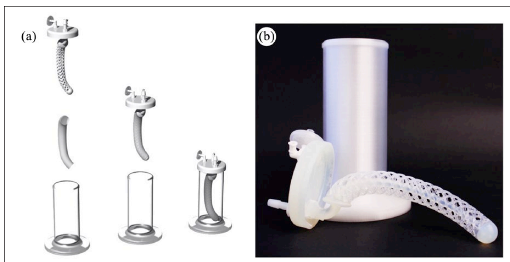
Figure 5. A custom patient-specific seeding apparatus was designed to accommodate the custom seeding mandrel. (a) Rendering of 3D-printed patient-specific closed-disposable seeding system. (b) Photograph of 3D-printed apparatus fabricated as a proof of concept.
