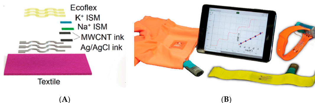
Figure 18. (A) Scheme of the manufacturing process on a polyurethane (PU) substrate. (B) Examples of use of the sensor, on underwear, wristband, and headband, illustrating the versatility of the printable and stretchable sensor array on different common wearable objects. The tablet displays a real-time trace of increasing potassium levels obtained wirelessly by the underwear printed sensor. Reproduced from [60] with permission. © 2016 WILEY-VCH Verlag GmbH & Co. KGaA, Weinheim.
