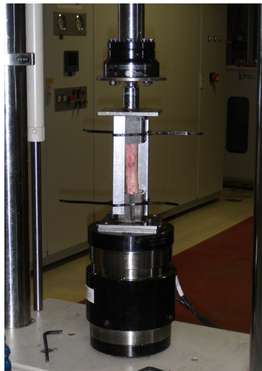
Fig. 1 The alignment phase of the experimental preparations necessitated the use of two right-angled supports to achieve alignment of the distal and proximal bone ends prior to securing with Wood's metal. Aligning the centroidal axis of the bone to the vertical ensured a consistent application of load across all samples
