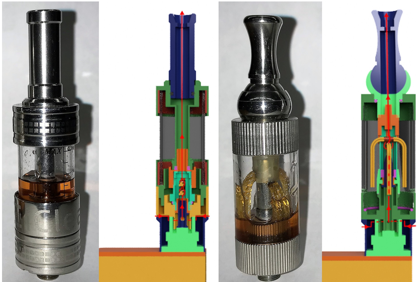
Fig 2. Comparison between the coil/wick designs for the two clearomizer tanks tested in this study. Shown are photographs and CAD renderings created by RIT engineers illustrating the differences in clearomizer designs for Innokin iClear X.I dual coil tank (left two panels) and the Innokin iClear 30 dual coil tank (right two panels). The hypothesis tested in this study is that the bottom coil Innokin iClear X.I with gravity-fed wicks would produce aerosol more effectively (e.g. with higher whole aerosol mass concentrations) than the Innokin iClear 30 upper coil tank with capillary-action-fed wicks.
