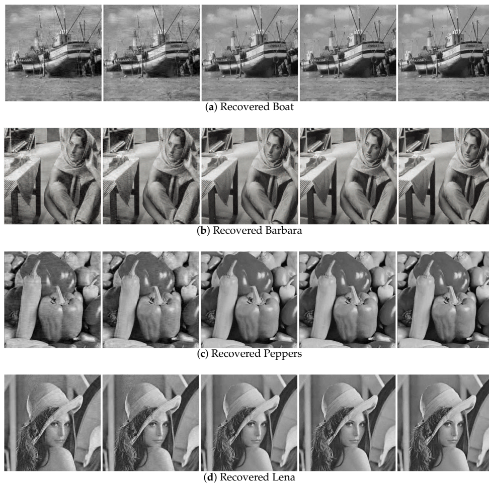
Figure 7. Image recovery effect by the BPDN, SL0, NSL0, L_p -RLS, and WReSL0 algorithms with noise intensity \delta_N = 0.01 . In (a–d), from left to right, are: image recovered by the BPDN, SL0, NSL0, L_p -RLS, and WReSL0 algorithms.
