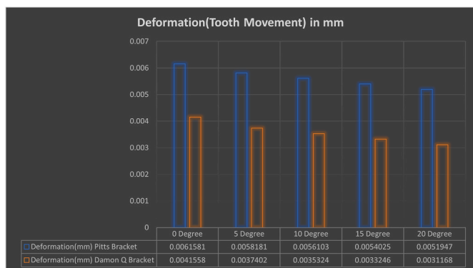
Fig. 4. Comparison of total deformation (tooth movement) with Damon Q and Pitts 21 at different inclinations.
