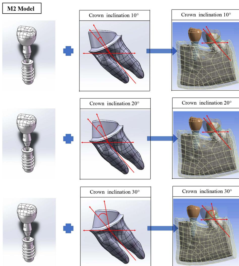
**Figure 2** Models (M2) with implant and three angles of crown preparation from the tooth root ( $10^\circ$ ,  $20^\circ$ ,  $30^\circ$ ).
