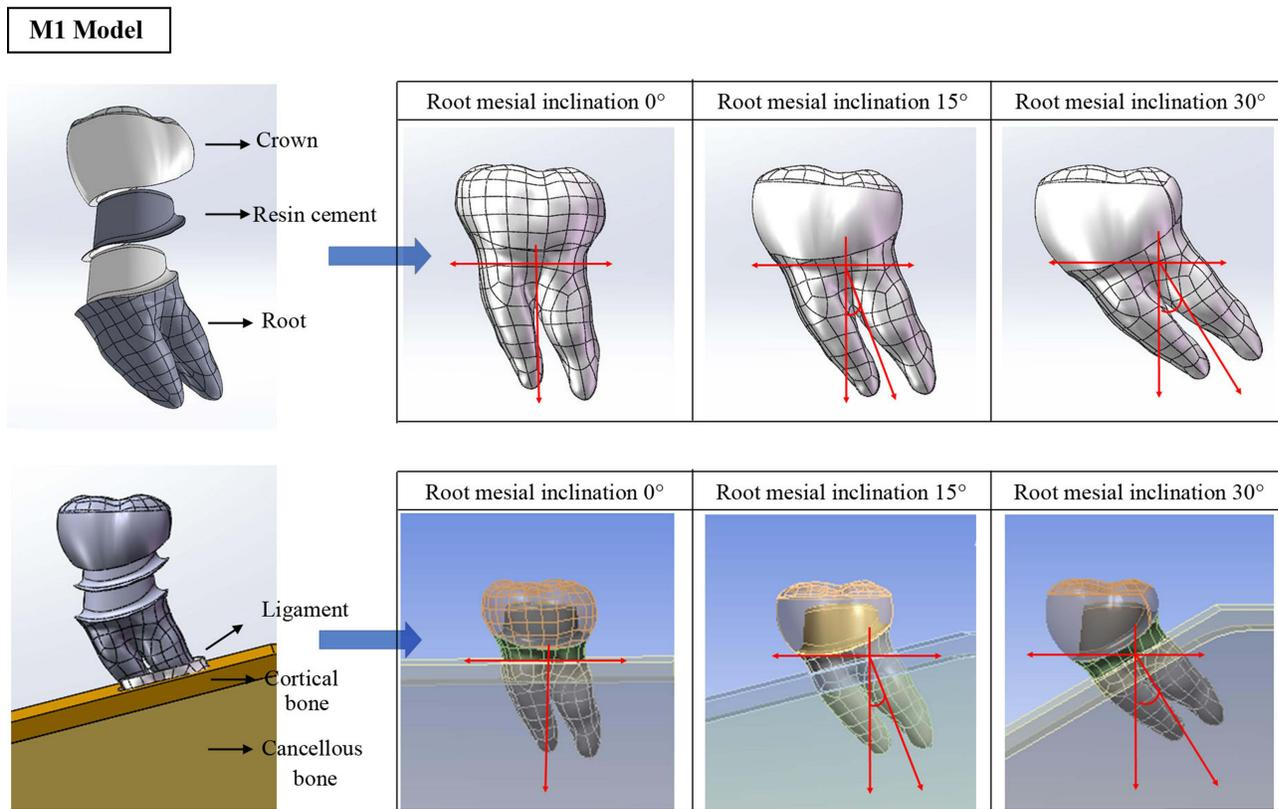
**Figure 1** Models (M1) with three angles of tooth root from the vertical direction ( $0^\circ$ ,  $15^\circ$ ,  $30^\circ$ ) and exploded view of simulation model design.
