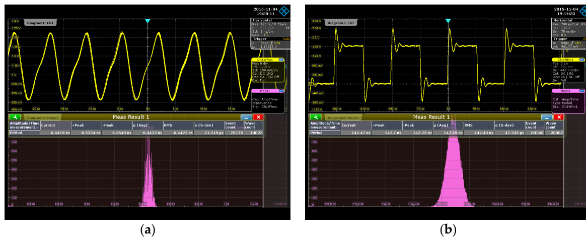
Figure 11. Jitter histogram at (a) 155 MHz and (b) 7 MHz.
