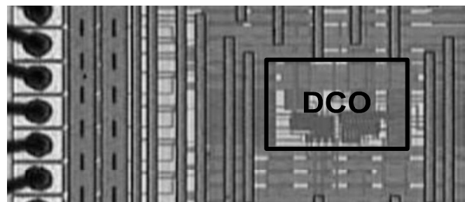
Figure 8. The chip microphotograph of the DCO chip.
