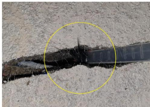
Figure 12. Rupture of textile (SN specimen).
