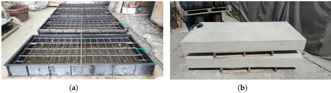
Figure 4. Fabrication of full-size slab specimens: (a) steel reinforcement; (b) cured specimens.
