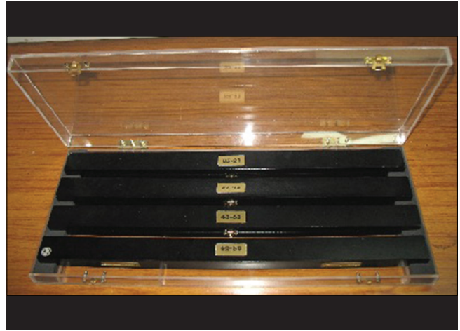
Figure 2: Our modified transparent carrier box for the FM-100 hue test
