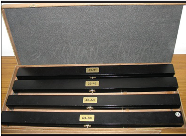
Figure 1: The original FM 100-hue elongated boxes with an opaque wooden cover
