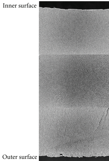
FIGURE 6: The scanning electron microscopy findings of cross-section structure of PMMA. PMMA has a symmetric structure having nearly homogenous microscopic pores from inner surface to outer surface of hollow fiber.
