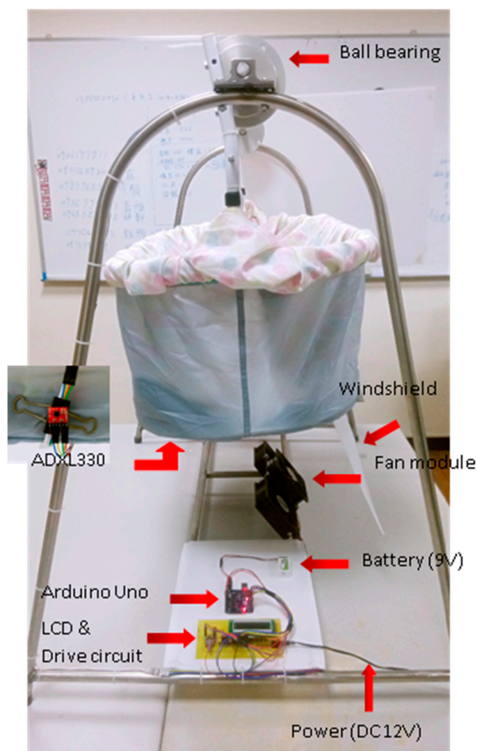
Figure 2. A resonant cradle design using wind power.
