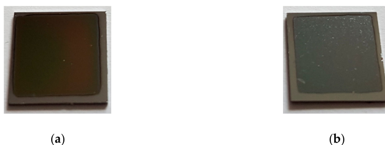
Figure 2. Macroscopic images of EVA_E (a) and EVA_L (b) films deposited on silicon wafer substrates.
