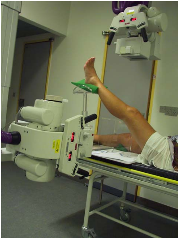
Fig. 1 Bi-planar RSA-setup with the two X-ray tubes at right angles and the patients right knee placed in the calibration knee cage. To gain overview scatter grids and X-ray film cassettes are not mounted
