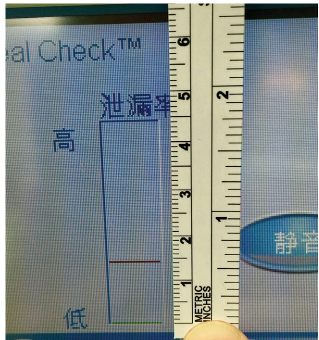
Fig. 1. Seal check on the NPWT device measured by a ruler. The total bar length is 45 mm and was converted to a 0–10 scale score.
