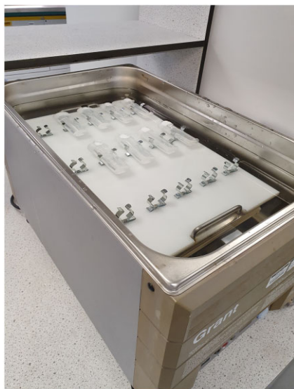
Figure 2020.07C. Polypropylene tube-holder in a Grant OLS 200 water bath to attach 40 mL polypropylene tubes containing samples.
