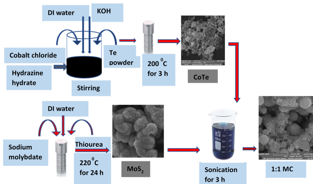
Scheme 1. Schematic illustration of MoS 2 , CoTe and MoS 2 /CoTe heterostructure formation.
