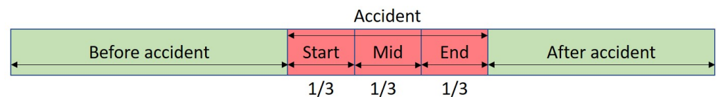
Figure 6. Temporal partition of the video. Dividing the accident part in three pieces of same length to evaluate the results by sections.
