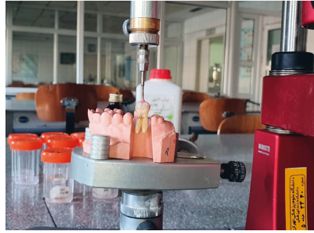
FIGURE 1: The process of mounting tooth specimen using a surveyor (the tooth is not in its final position).
