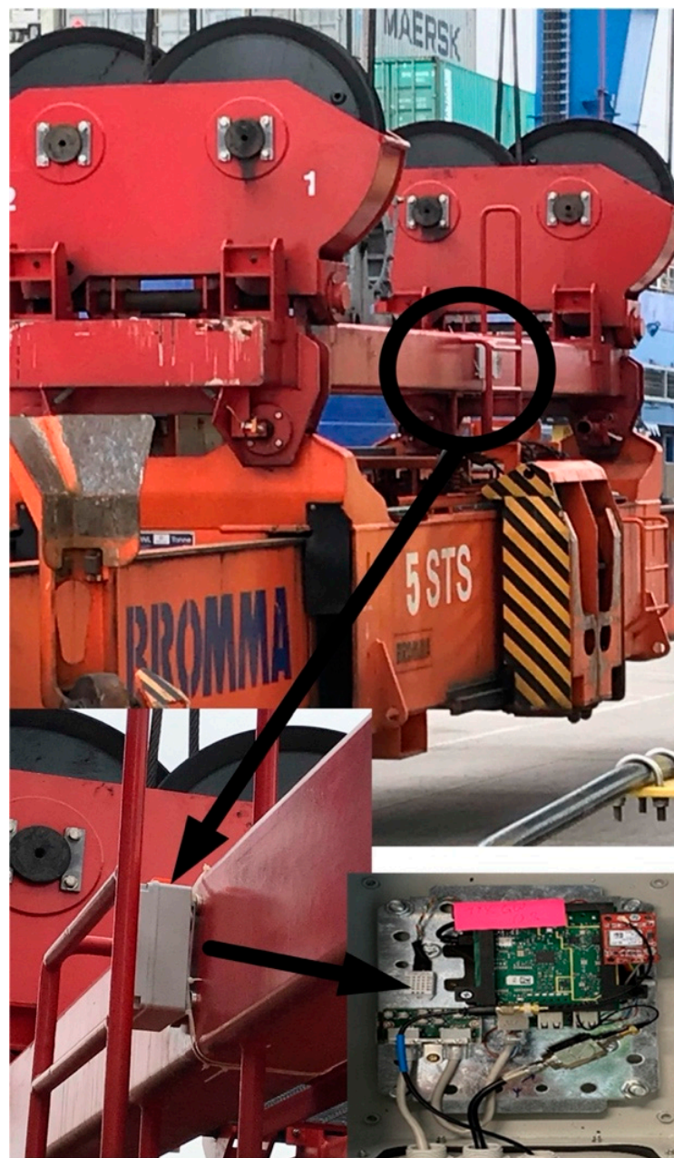
Figure 5. Positioning of the embedded sensory device on the spreader of the QC.
