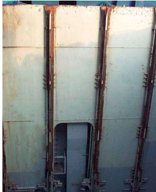
Figure 2. Example of the vertical cell guides in the inner hull of container ship representing the hold.
