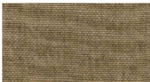
Figure 4. Sample of wool fabric dyed with 1% of the dye obtained through the LAC-mediated oxidation of ANS substrate.
