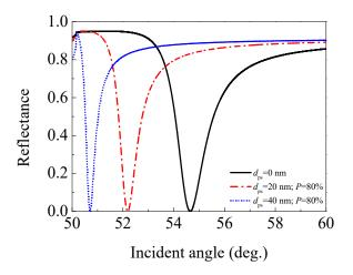
**Figure 7.** (Color online) The angular spectra of the SPR sensors with 0 (traditional SPR sensor), 20, and 40 nm thick 80% porosity porous silica film ( $n_{ps} = 1.086$ ).
