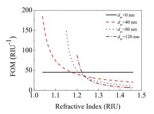
Figure 9. FOM versus the refractive index of porous silica film with various thicknesses.
