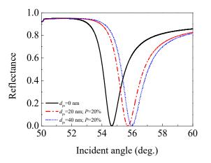
**Figure 4.** The angular spectra of the SPR sensors with 0 (traditional SPR sensor), 20, and 40 nm thick 20% porosity porous silica film ( $n_{ps} = 1.365$ ).
