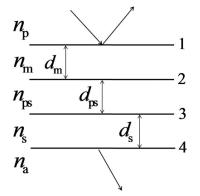
Figure 2. Three-layer model of the proposed SPR sensor.
