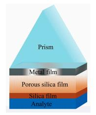
Figure 1. Schematic of the surface plasmon resonance (SPR) sensor with a porous silica film.
