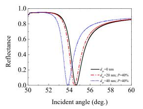
**Figure 5.** The angular spectra of the SPR sensors with 0 (traditional SPR sensor), 20, and 40 nm thick 40% porosity porous silica film ( $n_{ps} = 1.270$ ).
