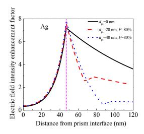
Figure 8. (Color online) Electric field intensity enhancement factor inside the SPR sensors in Figure 7.
