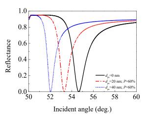
**Figure 6.** The angular spectra of the SPR sensors with 0 (traditional SPR sensor), 20, and 40 nm thick 60% porosity porous silica film ( $n_{ps} = 1.176$ ).
