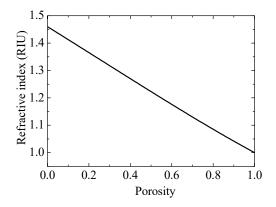
Figure 3. Refractive index as a function of the porosity of the porous silica film.
