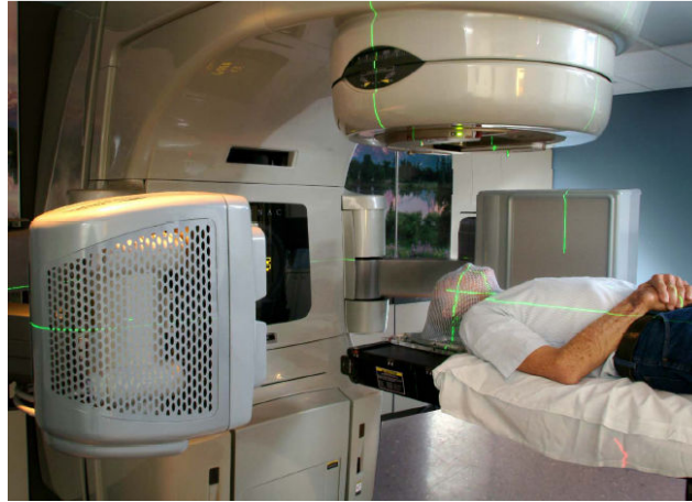
Figure 13 A linear accelerator with built-in kV cone beam CT system for IGRT treatment delivery (courtesy of Varian Medical Systems)
