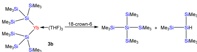
Scheme 2. Decomposition of Bis[tris(trimethylsilyl)silyl]ytterbium Complex 3b by Addition of 18-crown-6
