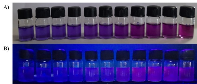
Figure 2. Sensing performance of the DDPT 1 (90 \mu M) in THF with the addition of trifluoroacetic acid (0.2 to 2 equiv.) A) under visible light B) under UV light illumination at 365 nm.
