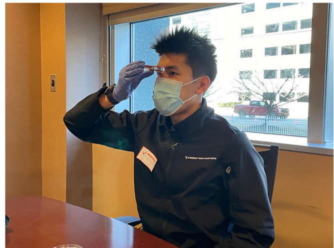
Figure 1 Subjects held the face mask scenario-specific plate to the bridge of their nose, facing downward and parallel to the floor.
