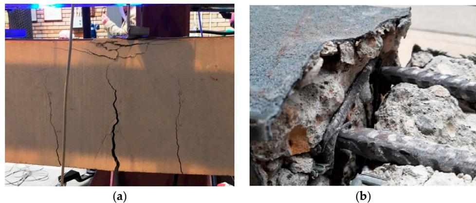
**Figure 14.** Failure mechanisms of the RC beams: (a) A beam without the polyurea coating; (b) A polyurea-coated beam.
