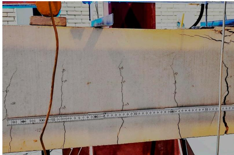
**Figure 11.** The cracking pattern captured by marking in RC beam.
