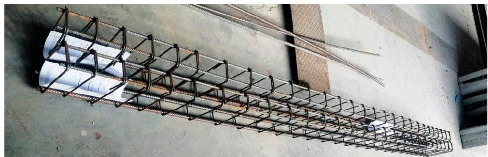
**Figure 3.** The arrangement of rebars for the RC beams before concreting.
