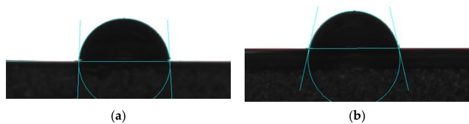
Figure 10. Photos of water contact angle of the control and ACP-treated samples. (a) Untreated soy protein film. (b) Soy protein film treated at 30 kV for 3 min. Untreated soy protein film was considered as the control. The amount of soy protein was 10% and glycerol was 2.8%.
