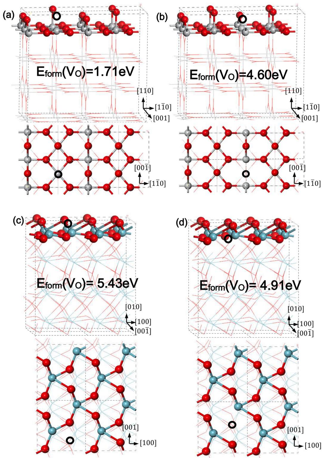
**Fig. 10.** Calculated structures (side and top views, respectively) of an isolated O vacancy at (a and b) the rutile  $\text{TiO}_2$  (110)- $2 \times 2$  surface and (c and d) the B- $\text{Nb}_2\text{O}_5$  (010)- $2 \times 2$  surface formed through removing the oxygen atom (i.e.  $\text{O}_T$ ,  $\text{O}_B$ ,  $\text{O}_{2C}$  and  $\text{O}_{3C}$ ) in (a), (b), (c) and (d), respectively. The circles illustrate the approximate positions of the isolated oxygen vacancies.
