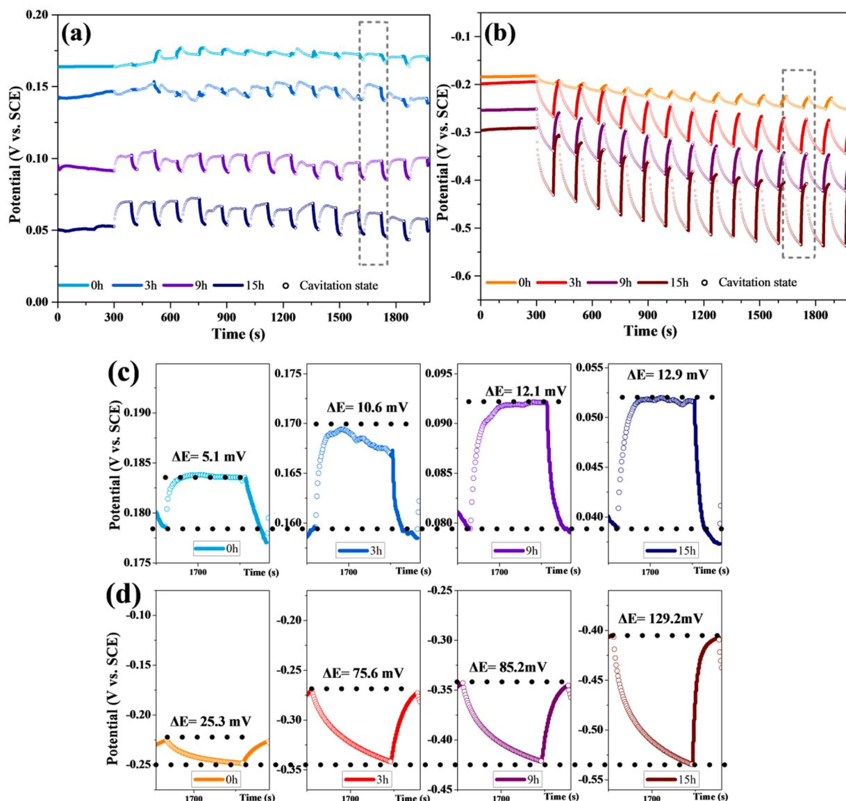
**Fig. 4.** The  $E_{OCP}$  vs. time plots for (a) the NbN coating and Ti-6Al-4V substrate (b) under the cavitation erosion cyclic conditions with the duty cycle of 75% (90 s ON and 30 s OFF) at an output power of 800 W in a 3.5 wt% NaCl solution. (c) The  $E_{OCP}$  vs. time plots for the NbN coating and the Ti-6Al-4V substrate for one cycle of cavitation erosion.
