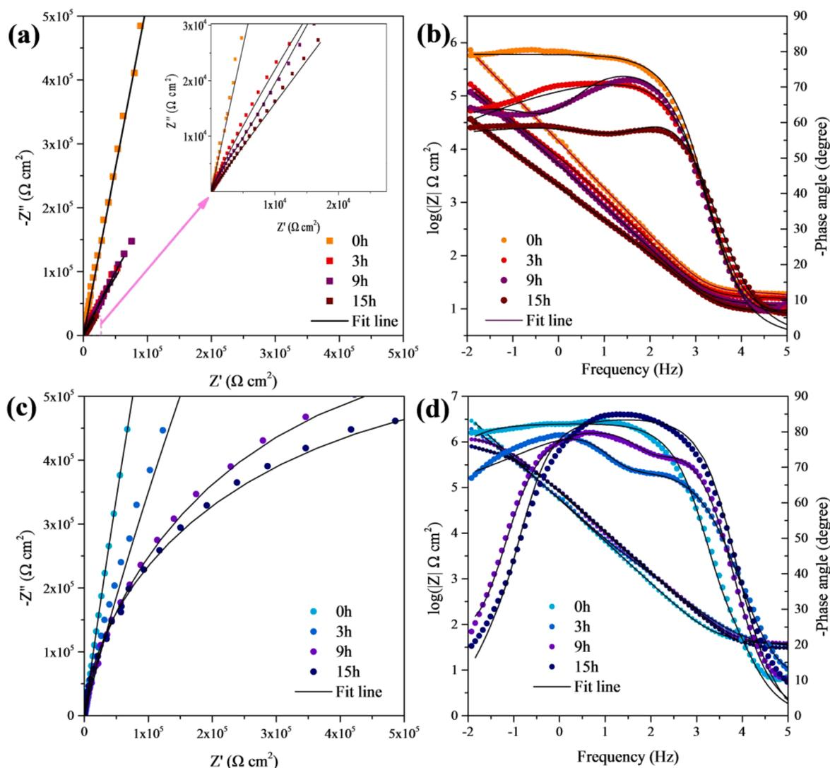
**Fig. 7.** (a and c) Nyquist and (b and d) Bode plots collected from uncoated Ti-6Al-4V and the NbN coating in a 3.5 wt% NaCl solution before and after different times of cavitation erosion with an output power of 800 W. (a and b) the NbN coating, (c and d) uncoated Ti-6Al-4V. The equivalent electrical circuits (e)  $R_s(Q_fR_f)$ , (f)  $R_s(Q_pR_p)(Q_bR_b)$  and (g)  $R_s(Q_o(R_o(Q_iR_i)))$  used for modeling experimental EIS data.
