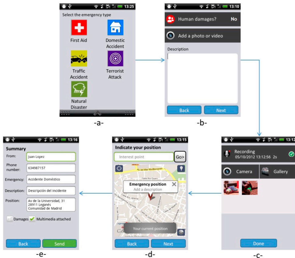
Figure 1. Application screen flow: -a- the emergency category list, -b- the textual description, -c- the multimedia content, -d- the localization map, -e- the message resume
