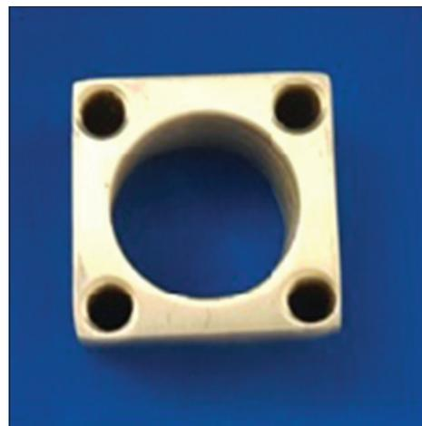
Figure 1: Custom made Stainless steel block 29 mm × 29 mm × 18 mm with a cylindrical mold space of diameter 23 mm and depth of 18 mm
