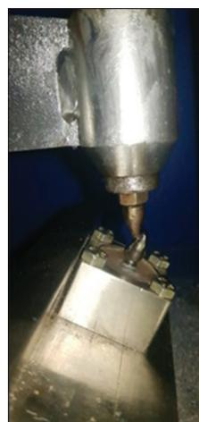
Figure 6: Cyclic loading of test samples with cemented Ni-Cr crowns
