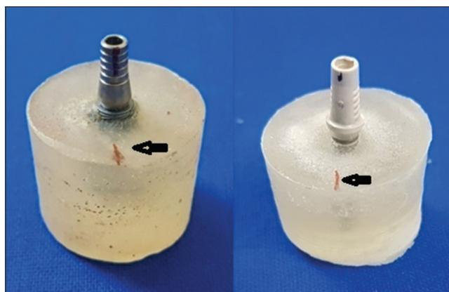
Figure 2: Placement of implant abutment assembly in a the stainless steel block and autopolymerizing resin pour
