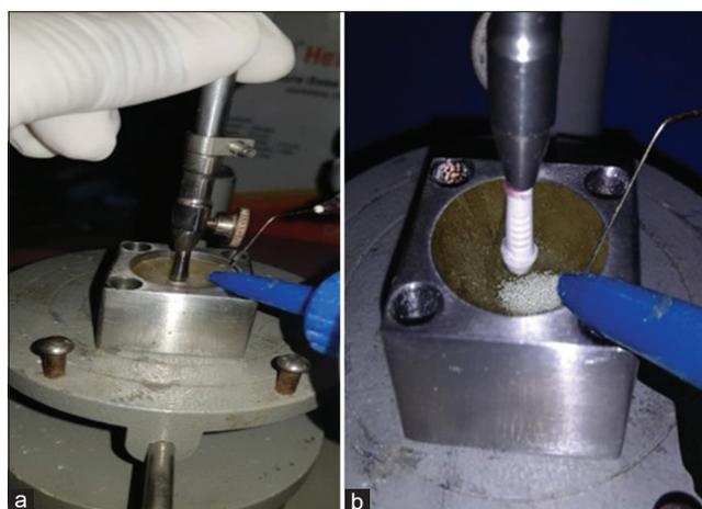
Figure 3: Implant abutment assembly with reference marks for reorientation in mounted resin blocks. (a) Titanium abutment, (b) Polyether ether Ketone abutment
