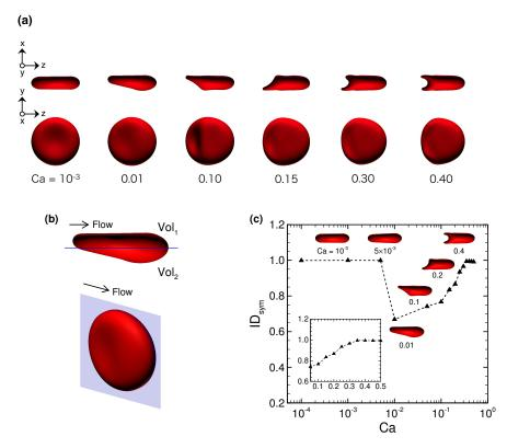
**Figure 3.** (a) Snapshots of a fully deformed RBC for different *Ca*. (b) Typical snapshots of a RBC at *Ca* = 0.01, where the blue plane denotes the center of the *x*-*z*-plane parallel to the flow direction, dividing the cell into the volume 1 (*Vol*<sub>1</sub>) and volume 2 (*Vol*<sub>2</sub>). (c) The symmetry index *ID*<sub>sym</sub> as a function of *Ca*. The insets represent snapshots of deformed RBCs at specific *Ca*.
