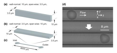
**Figure A1.** Detailed channel geometry. Magnified view of the channels with the cross-sections of (a)  $10 \ \mu m \times 3.5 \ \mu m$  and (b)  $3.5 \ \mu m \times 10 \ \mu m$ , which were used in Figure A2 and Figure A1, respectively. (c) Schematic view of the whole channel, whose stream-wise length was 8000  $\mu m$ . (d) Representative images of a flowing RBC in a microfluidic device. Flow direction is from left to right.
