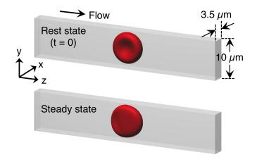
**Figure 1.** Computational domain to reproduce a translating red blood cell (RBC) in the narrow rectangular microchannel. The domain mimicked a microfluidic device as shown in Figure A1. The domain cross-section was 10  $\mu$ m  $\times$  3.5  $\mu$ m along the wall-normal and span-wise directions, respectively, and the stream-wise distance was set to be 50  $\mu$ m. Flow direction is from left to right.
