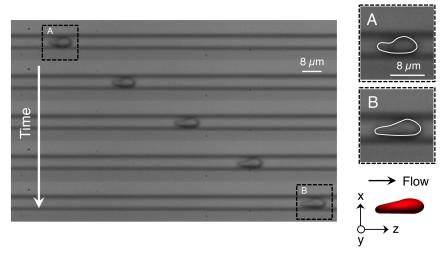
**Figure A2.** Representative images of the flowing RBC at frame numbers 0 (top), 20, 40 60, and 80 (bottom), respectively, where the speed of the cell is 1200  $\mu$ m/s (see also Video S1). A representative numerical result of a stable slipper-shaped RBC subjected to *Ca* = 0.01 (calculated centroid velocity  $V_c \sim 25 \mu$ m/s) is also displayed (see also Video S2).
