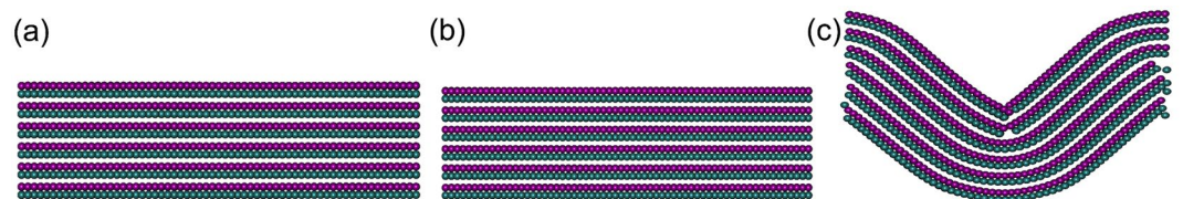
Figure 4. Snapshot of six-layer BP when compressing in the zigzag direction at selected compressive strains: (a) 0.000, (b) 0.020 and (c) 0.058.
