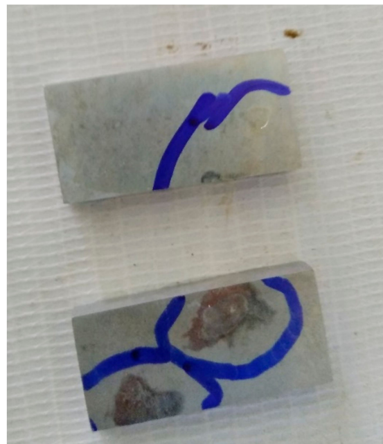
Figure 7. Corroded specimen after immersion test.
