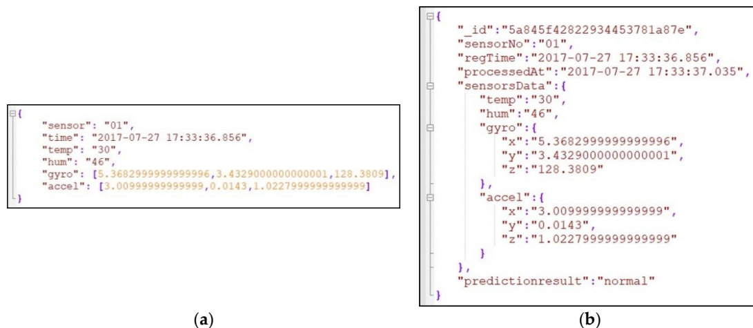
Figure 2. An example of sensor data generated by the IoT-based sensor presented in JSON format (a); and when stored in NoSQL MongoDB (b).
