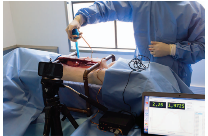
Figure 1. Experiment setup. The metal frame supporting the abdominal wall is in place with a camera positioned on a tripod. Punctures were performed every 1 cm with a hand sensor between the trocar and the surgeon's hand.
