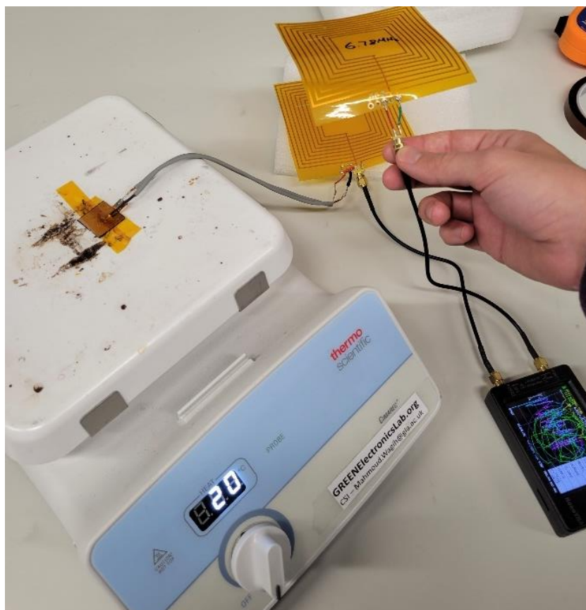
Figure S11. Photograph of NanoVNA wireless temperature sensing setup.
