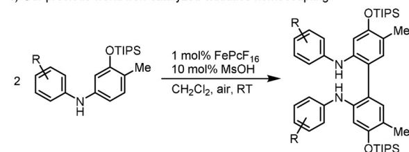
d) This work: iron-catalyzed oxidative cross-coupling with air as sole oxidant
