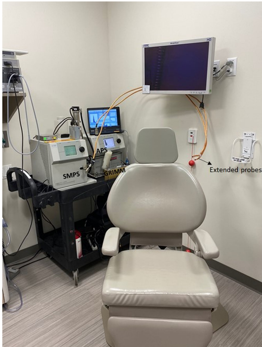
FIGURE 1 Setup of the aerosol measurement equipment in the clinic. Copper tubing was used to transfer the aerosols from near the patient to the SMPS and APS. Abbreviations: APS, aerodynamic particle sizer; SMPS, scanning mobility particle sizer
