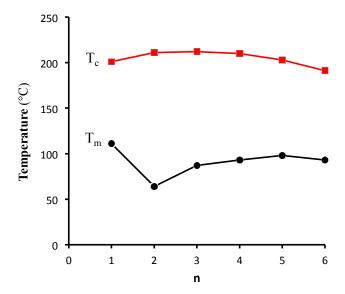
**Figure 6.** Plot of melting ( $T_m$ , black circles) and clearing ( $T_c$ , red squares) temperatures of linear alkyl esters  $2\mathbf{a} - \mathbf{f}$ , as a function of ester chain length, where n = # carbons in alkyl chain of ester (*i.e.*,  $2\mathbf{a}$ , n = 1;  $2\mathbf{b}$ , n = 2, etc.).
