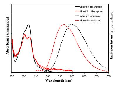
**Figure 2.** UV-visible absorption and emission spectra of 2a in solution ( $10^{-5}$  M CHCl<sub>3</sub>) and as thin films. Emission spectra were obtained using an excitation wavelength of 420 nm.
