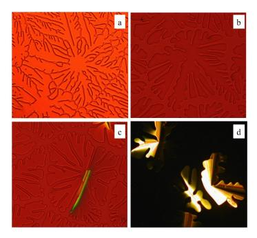
**Figure 4.** Representative polarized optical micrographs of columnar phases formed upon cooling from the isotropic phase of (a) **2b**; (b) **4**; (c) **6c** and (d) **7** (200× magnification). Images (a)–(c) viewed employing a 530 nm quarter wavelength retardation plate in order to improve viewing contrast.
