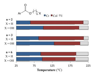
**Figure 7.** Phase ranges of compounds **2b**, **2c**, **2f** and **6a–c**; Cr = crystalline solid, Col = columnar hexagonal LC, I = isotropic liquid.
