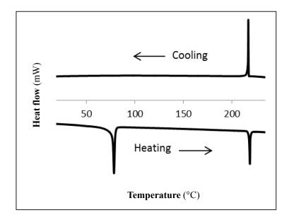
**Figure 3.** Differential scanning calorimetry (DSC) endotherm and exotherm for first heating and cooling cycle of 3 (heating/cooling rate =  $10 \, ^{\circ}$ C/min).
