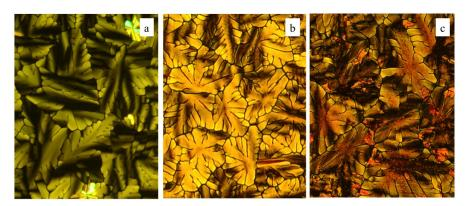
**Figure 5.** Polarized optical microscopy (POM) micrographs of compound **4** (**a**) at 175 °C; (**b**) at room temperature after 7 days and (**c**) at room temperature after 27 days.
