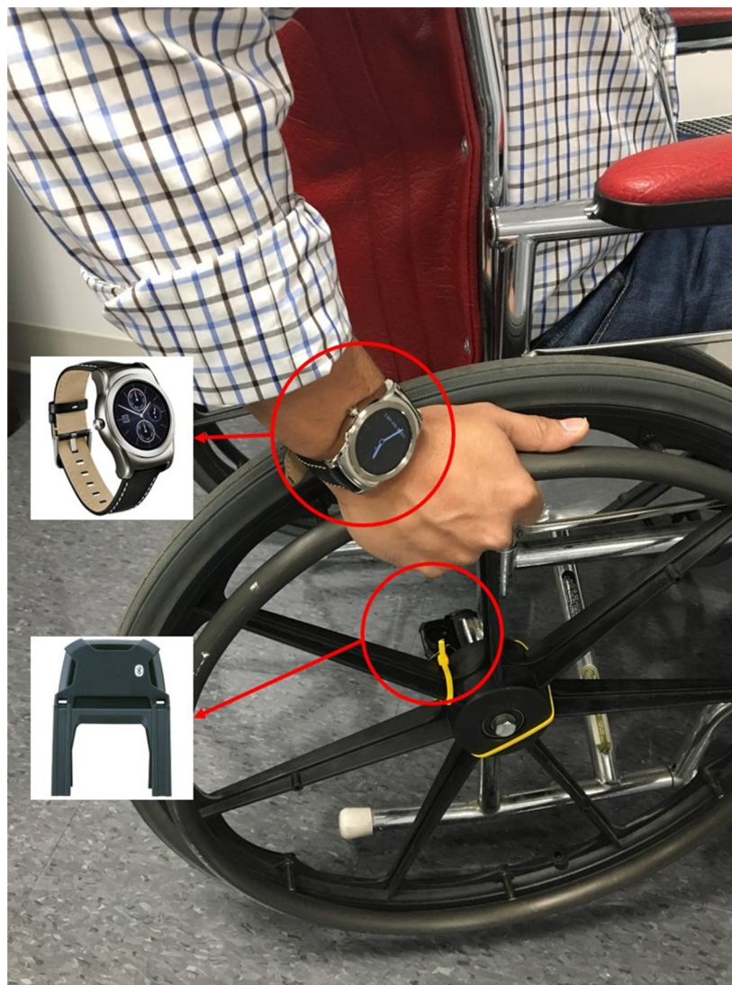
Fig 2. A participant using the JITAI sensors to measure and motivate PA.
