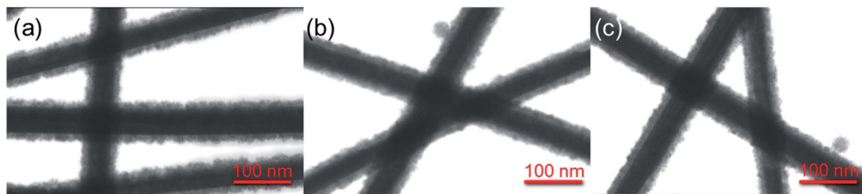
Fig. 2 STEM images of core/shell Ag/SnO 2 NWs (a) after the synthesis, (b) after 3 weeks and (c) 4 months kept in air at room temperature. The SnO 2 shell was obtained without microwave irradiation assistance.
